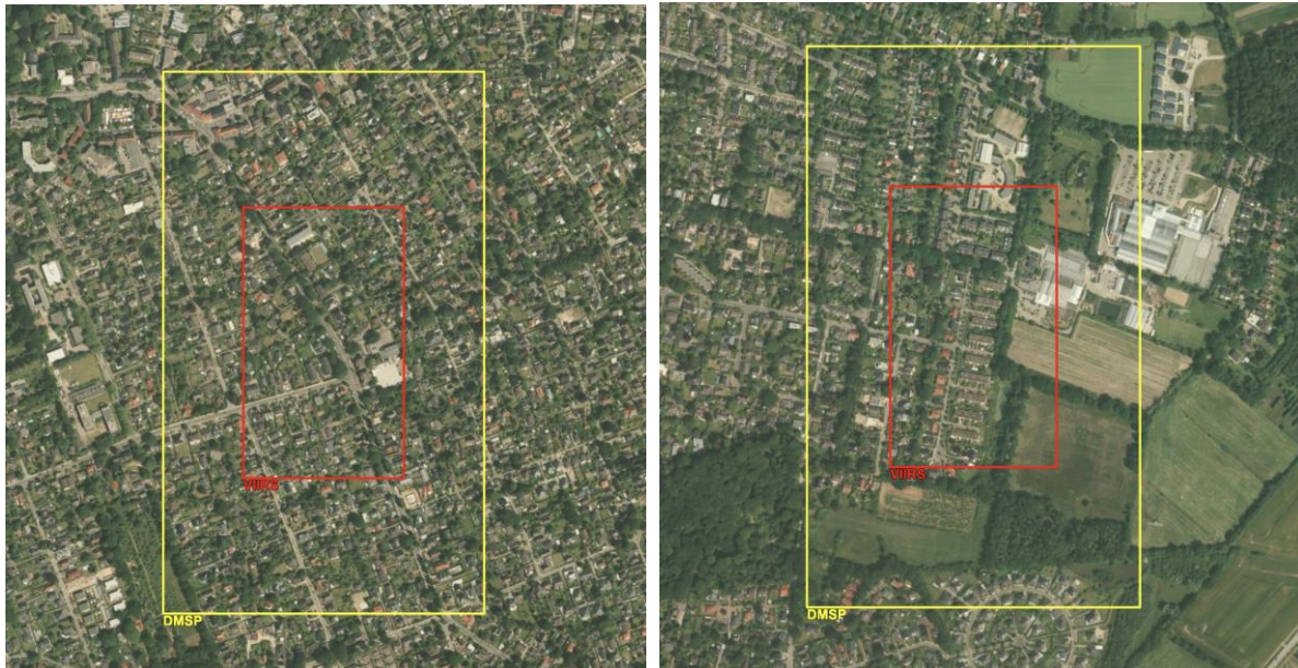
Fig. 7. Aerial imagery for two locations is shown with projected EOG pixels. The central (red) rectangle shows a reprojected DNB pixel, while the outer (yellow) rectangle shows the approximate size of a real DNB pixel. Note that in real operation, pixels will generally be tilted relative to North, and do not cover the same land area with each overpass (see e.g. Fig. 3 in Kyba et al., 2021). The figure is produced from screenshots of the Radiance Light Trends app (Stare & Kyba, 2019), and the background imagery is based on Bing Maps.
