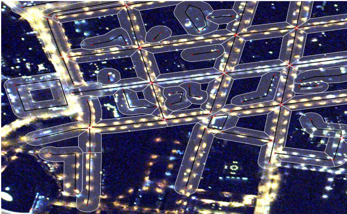
Fig. 14. A comparison of the areas counted in Potsdam's city center to nighttime aerial imagery. The transects shown here are from the bottom leftmost region in Fig. 9, and they are shown with a buffer to indicate the nearby areas. There are some regions with lights between the streets that were likely not counted as part of the surveys.
