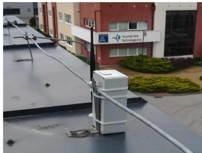
Fig. 1. A device measuring the brightness of the sky, placed on one of the TARR buildings in Toruń (Poland) (photo by Mieczysław Kunz, 2020)
