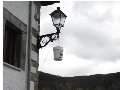
Fig. 1: One of the interception traps used to capture flying insects attracted to ALAN in the Western Pyrenees.
