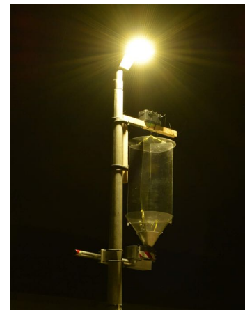
Fig. 1: Street-light (4000K) with an automated insect trap (Photo: Martin K. Obrist, WSL)
