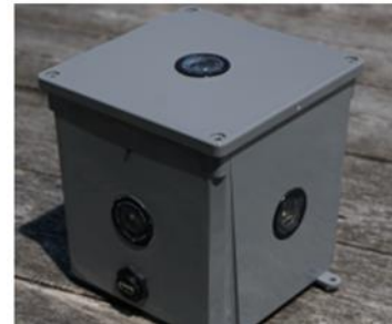
Fig. 1: A LAN3, a multispectral and multiangular nightlight sensor
