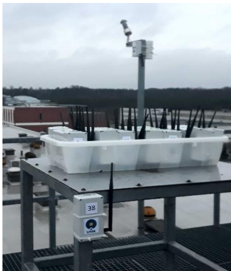
Fig. 2. Testing the cloud of devices for measuring the sky brightness in November 2020 on the terrace of the NCU Meteorological Observatory in Toruń (Poland), (photo by Mieczysław Kunz, 2020)
