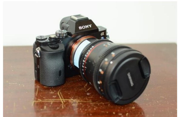
Figure 1. DSLR camera used to test the calibrating method. Sony a7s equipped with a Samyang T1.5 50mm lens. Photo credit: Alexandre Simoneau
